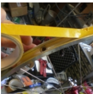
Photo 3: Applying tape over the glued rim bed.
